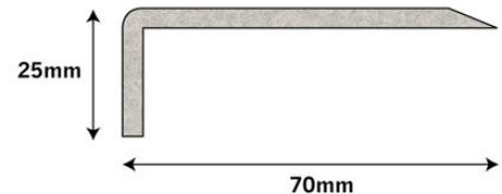
They have been slip resistance tested to AS 4586:2013 passing with the highest slip resistance rating of Class P5 for Wet Pendulum Test and Class DI for Dry Floor Friction Test - LRV values on request
