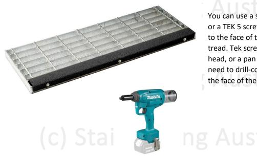
You can use a stainless steel TEK 3 or a TEK 5 screw to fasten the FRP to the face of the welded steel tread. Tek screws come with a Hex head, or a pan head. You would need to drill-countersink holes in the face of the FRP first.
