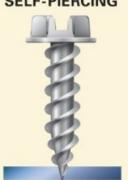
Self-piercing screws are engineered for use with light gauge metal and don't need a pilot hole. The high-strength fastener penetrates the metal and taps its own threads as it is driven into the material.
